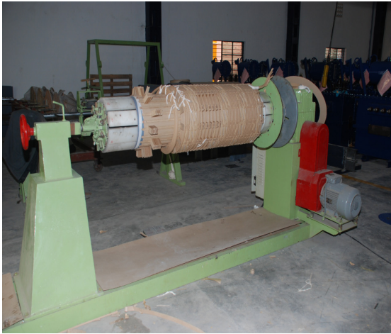
In house Winding Machine's up to 10 MVA
